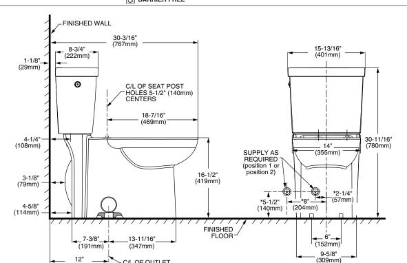
NOTES: THIS COMBINATION IS DESIGNED TO ROUGH-IN AT A MINIMUM DIMENSION OF 305MM (12") FROM FINISHED WALL TO C/L OF OUTLET. \* DIMENSIONS SHOWN FOR LOCATION OF SUPPLY ARE SUGGESTED. SUPPLY NOT INCLUDED WITH FIXTURE AND MUST BE ORDERED SEPARATELY.
