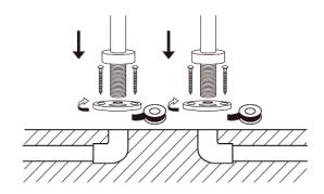
2. Wrap threaded ends of Bath Supplies (2) with teflon tape and thread through Cover Plates (4). Secure Cover Plates(4) to floor with Screws (5) provided. Thread enough through floor to ensure water connections can be done while testing height to ensure proper placement of tub filler over tub rim. Slide Floor Escutcheons (3) down to conceal Cover Plates.
