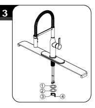
Secure the faucet assembly with the washers (1&2) and nut (3). Hand tighten the nut (3) onto the faucet assembly. Lock the nut (3) into position by tightening the screws (4) with a phillips screwdriver.
