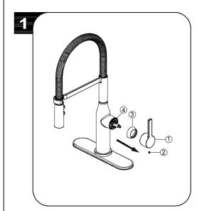
Shut off water supply. With valves in "closed" position, loosen the set screw (2) and remove handle (1). Unscrew the cap (3) from the cartridge nut (4).
