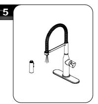
Important: after installation is completed, turn on hot and cold water supplies. Check for leaks. Remove the spray head by unscrewing it from the hose counterclockwise. Be sure to hold the end of the hose down into the sink and turn the faucet on to the warm position where it mixes hot and cold water. Flush water lines for one minute. Check for leaks. Re-tighten any connections if necessary, but do not overtighten. Reinstall spray head by hand tightening it back onto the spray hose.
