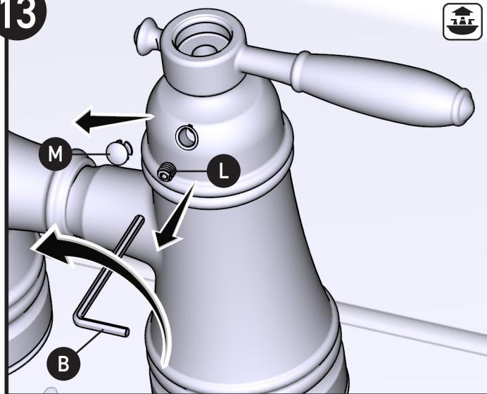
Remove Plug Button (M) (x2) and Set Screw (L) (x2) with 3/32" Hex Wrench (B).
