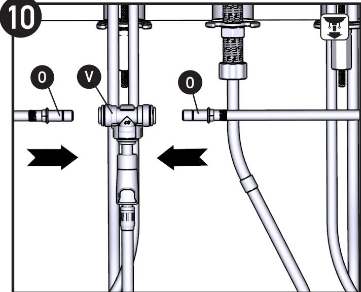
Install Outlet Hoses (**O**) (x2) into Adapter Tee (**V**).
