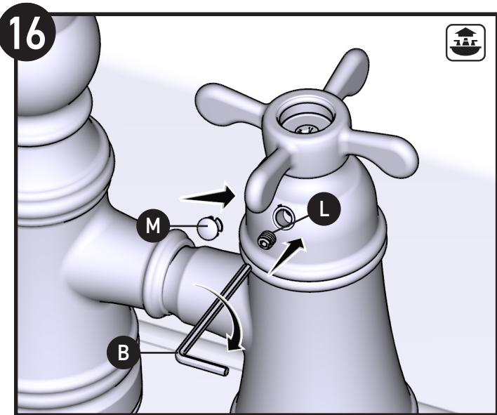
Install Set Screw (**L**) (x2) with 3/32" Hex Wrench (**B**) and then install Plug Button (**M**) (x2).
