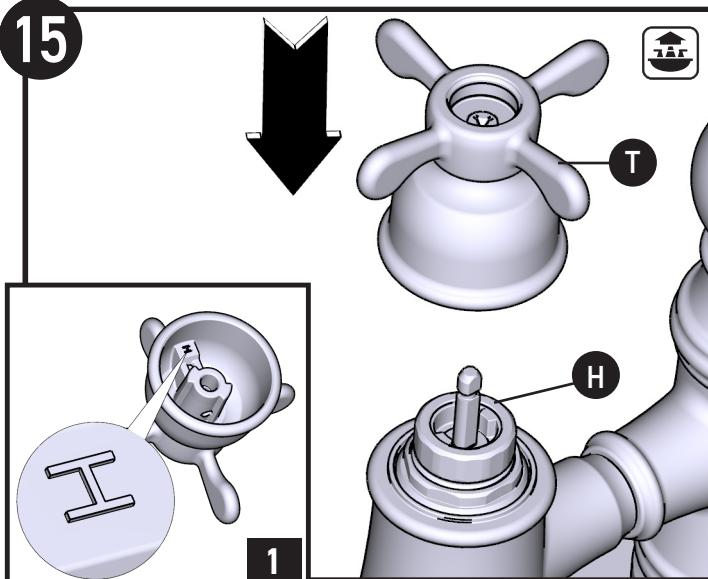
Install Alternate Handle (T) (x2) onto Handle Receptor (H) (x2). Ensure Hot Handle and Cold Handle are in correct positions.
