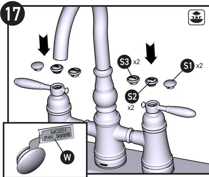
Choose Handle Cap style (**S1, S2, or S3**) (x2) and apply a small amount of Lubricant (**W**) to backside of Handle Cap (**S**). Attach Handle Cap (**S**) to Handle top.
