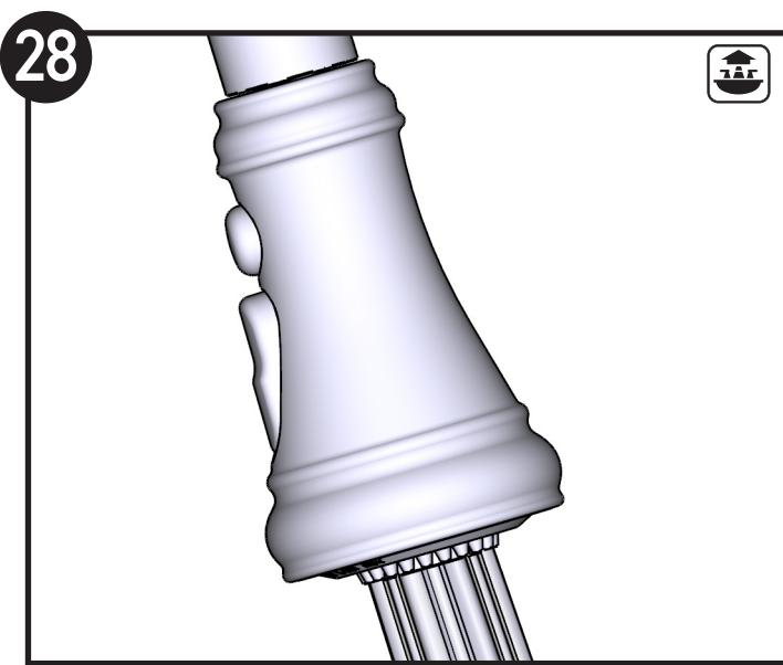
Reinstall screen and o-ring as shown. Thread Pulldown hose (**Q**) onto Spray Wand (**R**) and tighten as shown.
