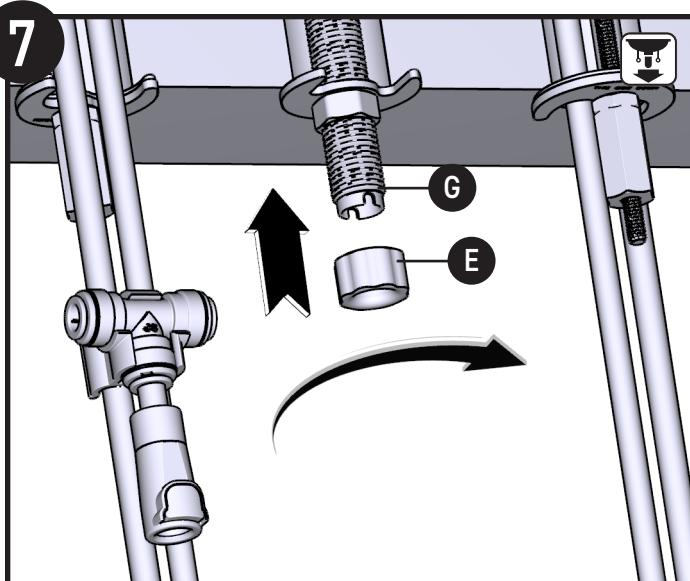
Install Hose Protector (**E**) onto Faucet Body (**G**), finger tighten.
