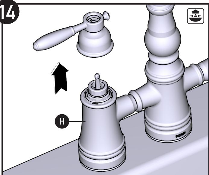
Remove Handle (x2) from Handle Receptor (H) (x2).
