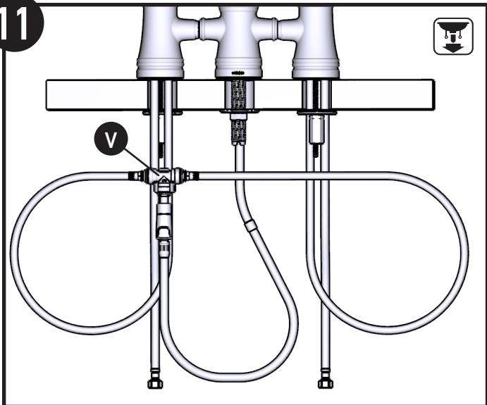
Hose installation into Adapter Tee (**V**) complete.
