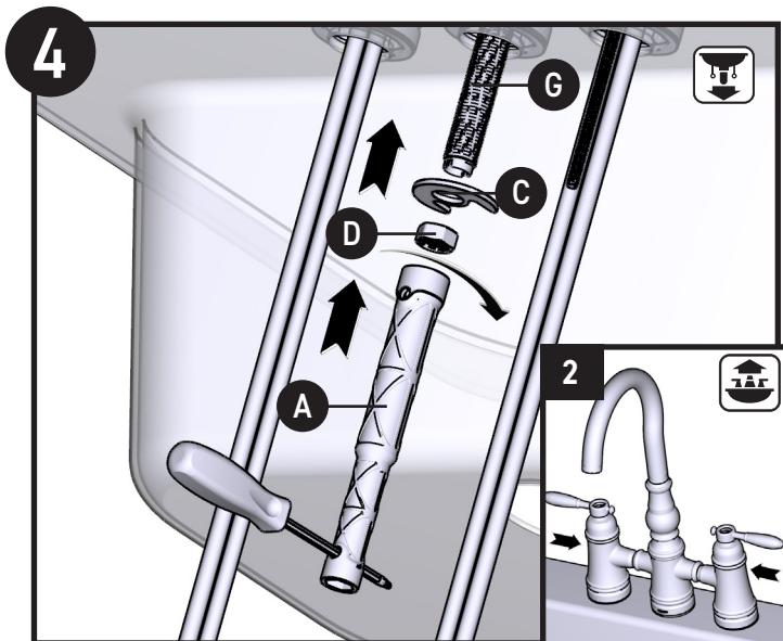
Using the installation tool (**A**), install Mounting Washer (**C**) and Mounting Nut (**D**) onto Faucet Body (**G**). After installing the mounting washer and nut, ensure the handle receptors are fully engaged into the faucet body.
