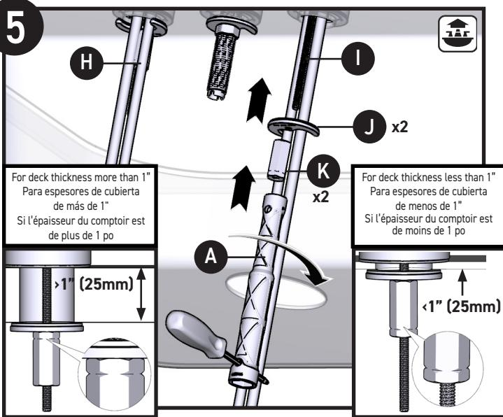
Using the Installation Tool (**A**) install the Handle Receptor Mounting Washer (**J**) (x2) and the Handle Receptor Mounting Nut (**K**) (x2) onto the Handle Receptors (**H**) and (**I**).
