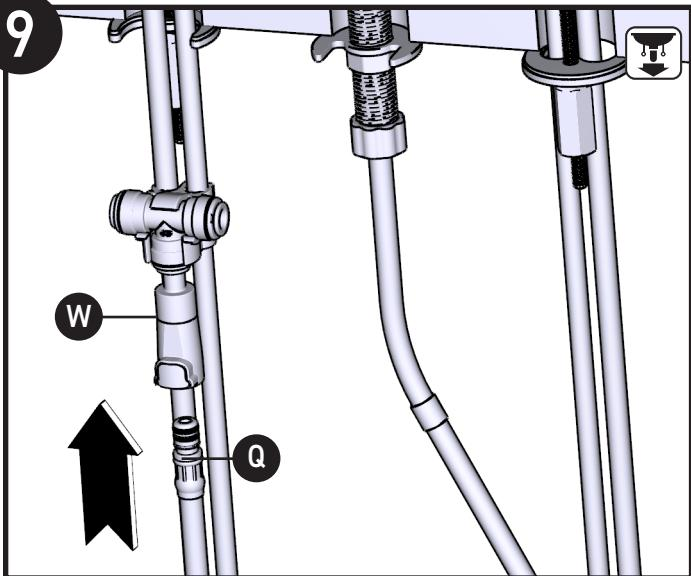
Insert Pulldown Hose (**Q**) into end of Hose Adapter (**W**). Push until a "click" is heard. Tug downward to test engagement.
