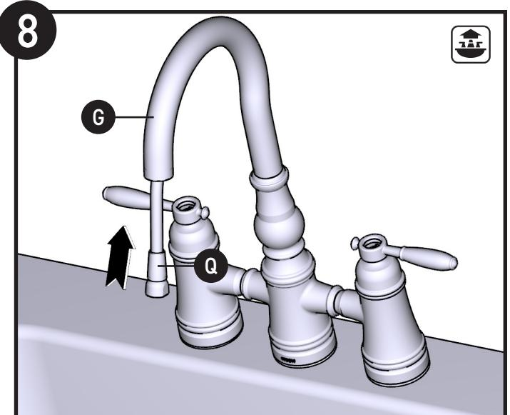
Insert small end of Pulldown Hose (**Q**) into spout and feed through Faucet Body (**G**). Twist the hose to overcome any resistance during installation.
