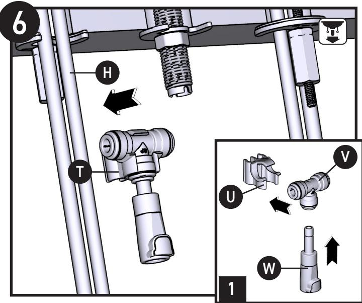
Clip Adapter Tee (**V**) into Adapter Bracket (**U**). Insert Hose Adapter (**W**) into Adapter Tee (**V**). Clip Adapter Tee onto Handle Receptor Hose (**H**).
