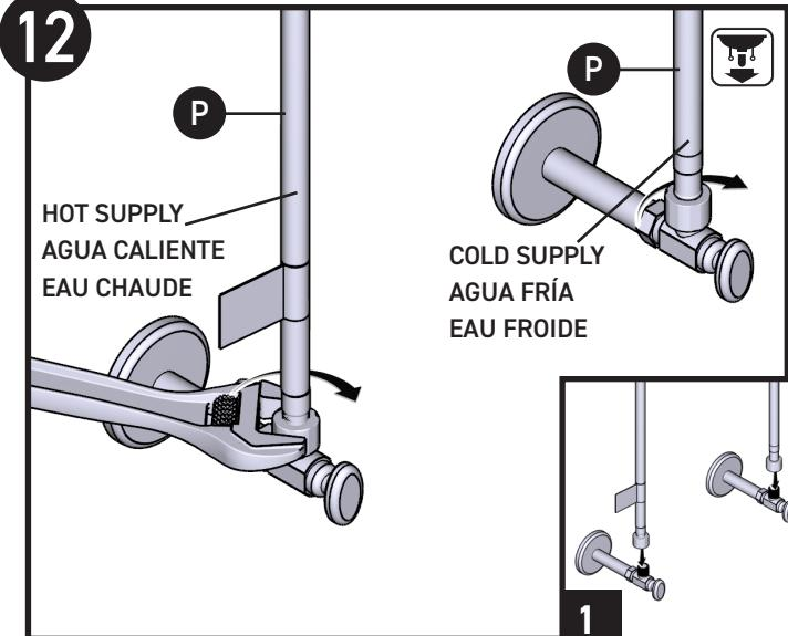
Attach Supply Hoses (**P**) (x2) to shut-off valves. Tighten with wrench until secure.
