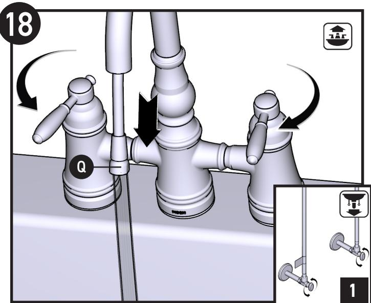
Turn on Hot and Cold water supply. Hold Pulldown Hose (**Q**) and turn on Faucet. Allow water to run 15 seconds.
