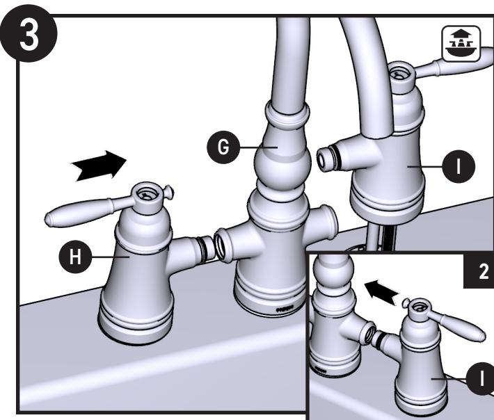
Install Handle Receptor (**H**) (hot) into Faucet Body (**G**). Install Handle Receptor (**I**) (cold) into Faucet Body (**G**).
