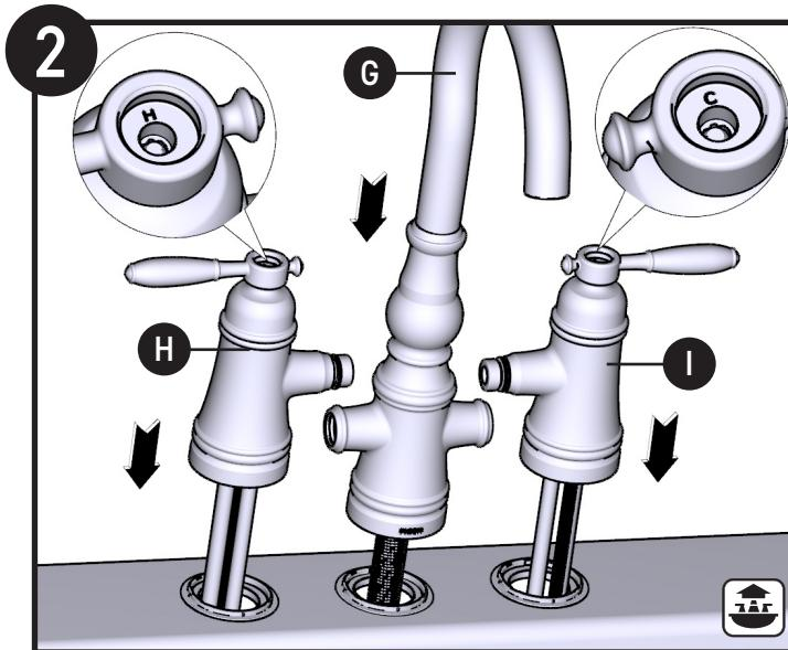
Install Faucet Body (**G**) and Handle Receptor (**H**) (hot) and Handle Receptor (**I**) (cold) onto sink.
