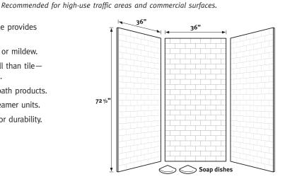
Designed to fit base areas 36" deep or smaller x 36" wide x 72-1/2" high or smaller (914 mm x 914 mm x 1829 mm)
