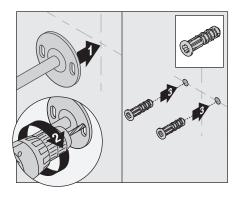
2b) **Stud Option:** Place mounting brackets into desired position. Using brackets as a guide, carefully drill 3/16" holes into wall.
