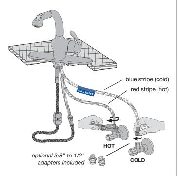
Step 6 Flush supply lines and check for leaks
