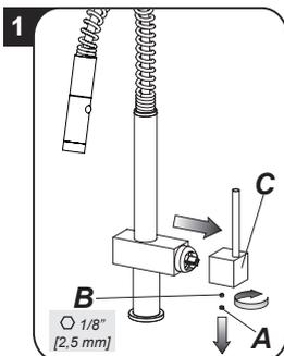
Before disassembling the faucet be sure that the water supply is turned off.
