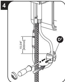
Attach the counterweight (D2) to the flexible hose approximately 15-3/4" [400mm] from the connection to the outlet pipe.
