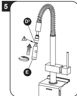
Tighten the shower (E) to the hose interposing the gasket (D3) and confirm the hose can slide smoothly through the passage hole.
