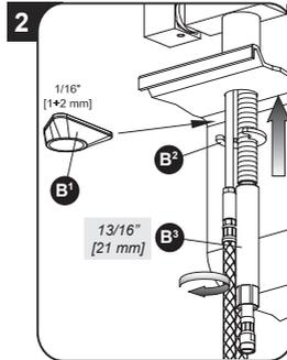
For countertop thicknesses less than 1/16" thick use the flange (B1), for all other installations use the metal washer (B2). Secure mounting hardware in place by tightening mounting nut (B3).
